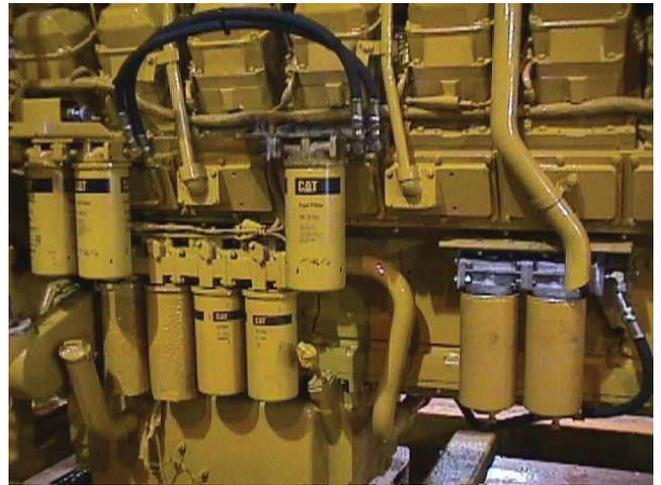
*Figure 10. Recommended Heavy Duty Onboard Filtration Arrangement, Circa 1998*
