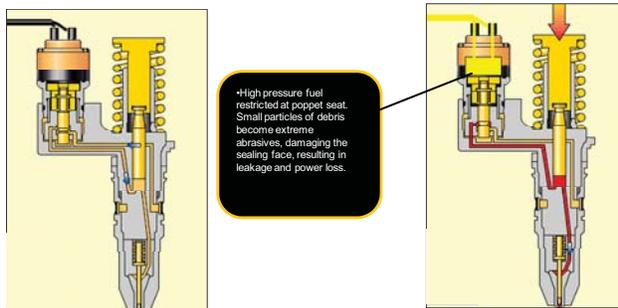
Figure 5. Caterpillar EUI Injector
