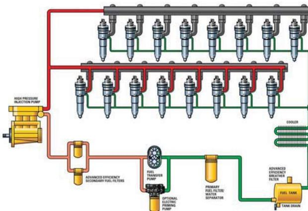
Figure 8. Typical Common Rail Fuel System
