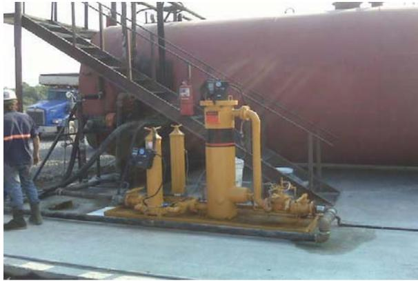
**Figure 15. Bulk Fuel Filtration Test at the White Flame Mine — Particle Detectors were Connected to the Inlet and Outlet Sampling Valves for Dynamic Testing.**
