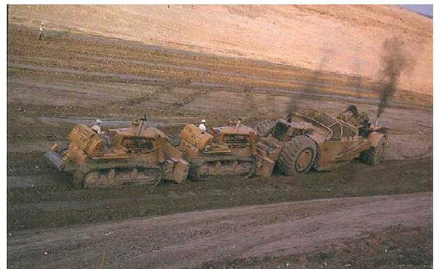
*Figure 4. Black Smoke Was a Sign of Power for Early Pump and Lines Fuel Systems*
