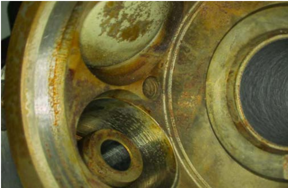
Figure 7: Metal housing of common rail pump with iron formate deposits 16
